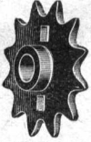
Nr. H 1532/1600 Für Sturmey-Archer \frac{1}{2} \times \frac{1}{8} " 12 Zähne b1 = 12,8, b2 = 10,5 H = 12,5, h1 = 9,5, n1 = 18 RM 20.—
