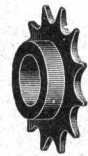
Nr. H 1458/1600 Für Fenag \frac{3}{8} \times \frac{1}{8} " 15 Zähne b1 = 13, b2 = 11 H = 10,1, h1 = 4,9, h2 = 22 n1 = 24,1, n2 = 23 RM 20.—
