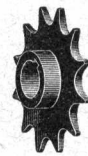
Nr. H 1440/1600 Für Bosch \frac{3}{8} \times \frac{1}{8} " 15 Zähne b1 = 10,7, b2 = 8,2 H = 12,2, h1 = 5,6, h2 = 3,7 n1 = 20,3, n2 = 20,3 RM 20.—
